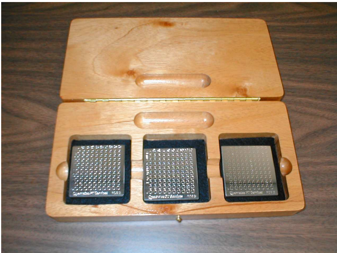
Fig. 1 Photograph of PT Artifacts for Rockwell Hardness
